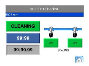
A push on the cleaning button will automatically launch a rinsing through the nozzles during the time set by the user. The activation of one or/and the other nozzle is up to the user.
