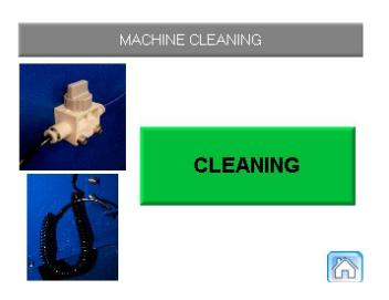
To launch a machine cleaning, you only have to open the tap shown on the first picture, to unroll the hose and to push « cleaning ». At the end of the cleaning, the user will have to close the tap.
